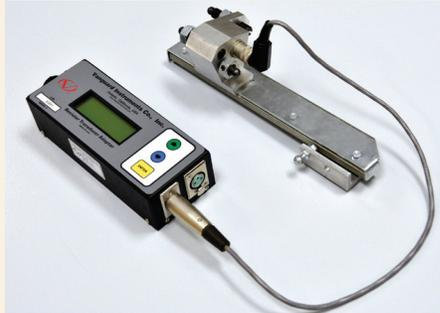
Connected to an ABB AHMB resistor-type transducer
